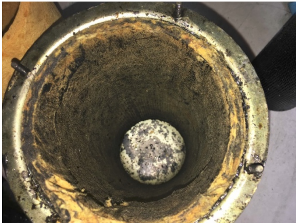
Image of filter basket and element showing excessive contamination in the form of TEG.
