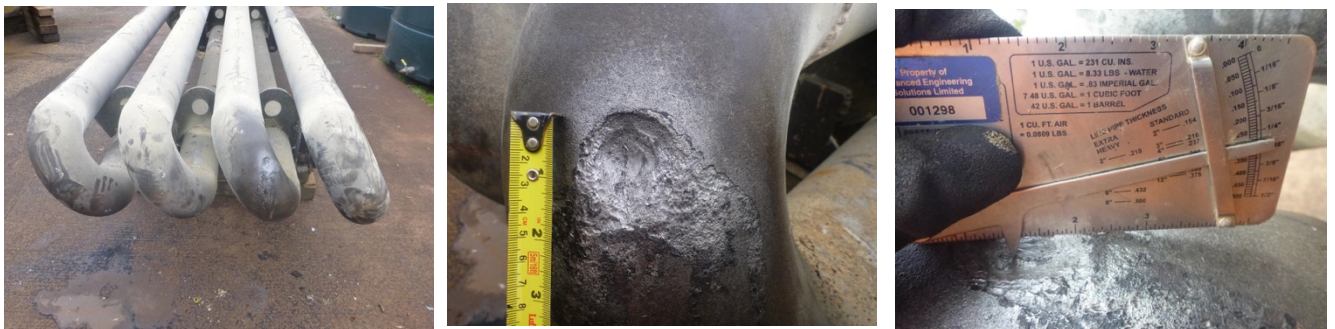
Images showing Weston Point Gas Coil Defect 1,2,3
