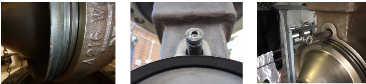
Images showing failure of piston tab on ERS Regulator at Didcot AGI
